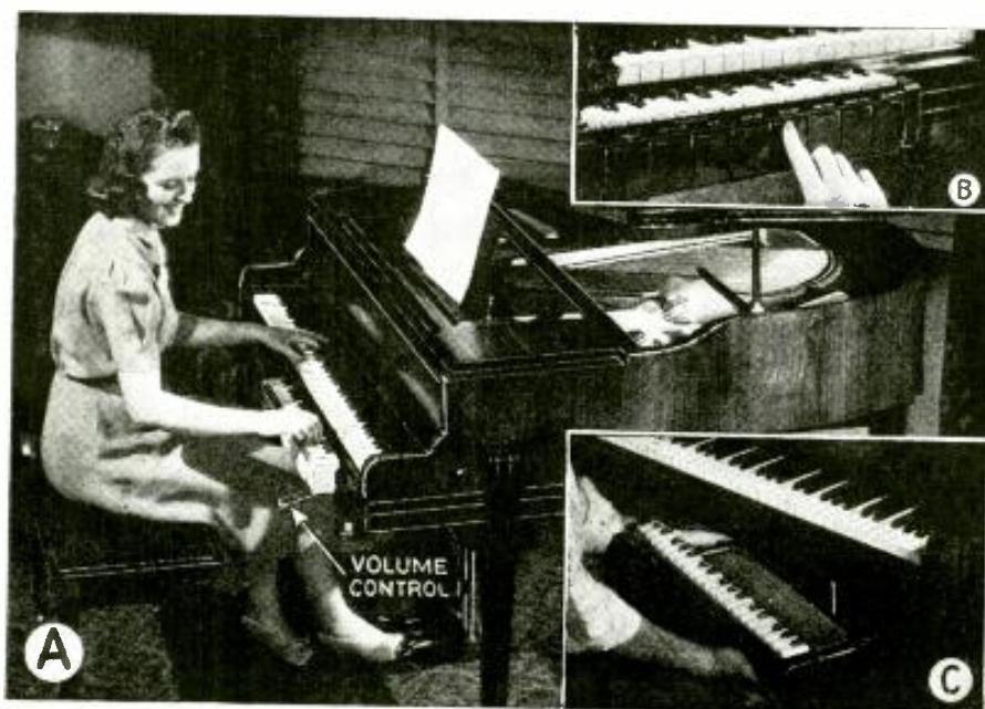
◀ The photos at left illustrate various elements of the Solovox. At A, the attachment in use on a grand piano, a set of 12 control tablets giving any piano an indefinite variety of tone colors that simulate the organ (Note individual volume control.); B, close-up of upper portion of the Solovox showing how the control tablet add-on device is tilted to produce a desired effect; C, the Solovox keyboard being attached to the piano keyboard by thumbscrews.
